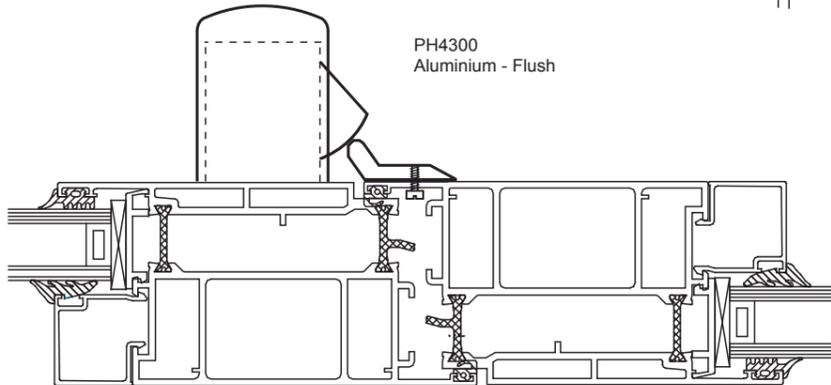
Floor strikers should be mounted on floor as shown. If aluminium low threshold strips are used the striker should be notched into aluminium section to comply with current legislation.
