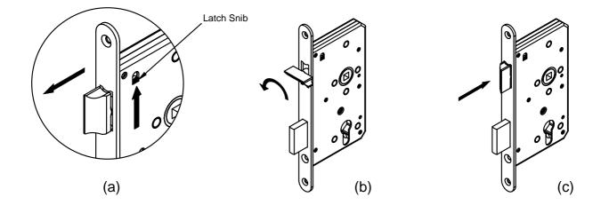
1) Release the latch head from the forend by pushing up on the latch snib. (a)
