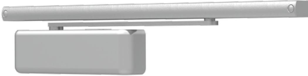
The 4030T is a single lever (track) arm, surface mounted closer designed for interior use on narrow head frames and top rails. The choice of three mountings and ease of installation offer a versatile solution to door control in moderate traffic applications. The 4030T compliments the heavy duty 4000 Series.
