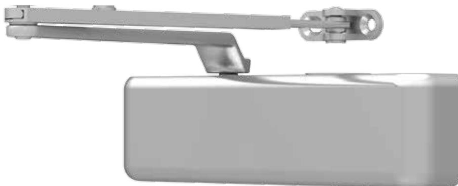
The 4030 is a cast iron, universal closer designed specifically for doors in moderate traffic conditions. This versatile closer compliments the rest of the heavy duty 4000 Series and offers the choice of three mountings and multiple arm options.
