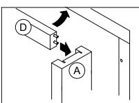
SLOT CROSS PIECE "D" TO THE ALREADY FITTED JAMB "B", FIX IN JAMB "A" , CHECK HIS VERTICAL POSITIONS AND FASTEN TO THE FRAME.
