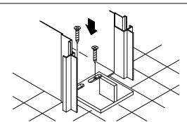
FIX FLOOR GUIDE USING SCREWS 4.2X9.5. IF THE FRAME IS NOT AT THE SAME LEVEL OF THE FLOOR USE THE SUPPLIED SPACER FOR THE FLOOR GUIDE AND IN THIS CASE USE SCREWS 4.2X19.
