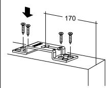
FIX THE BRACKETS, WHICH SUPPORT THE HANGERS, TO THE TOP OF THE DOOR AT 170 mm AS SHOWN IN THE DRAWING WITH 4.5X25 SCREWS. IT IS IMPORTANT THAT THE SLOT FOR HANGER HOOKING IS TOWARDS THE FRONT SIDE OF THE DOOR.
