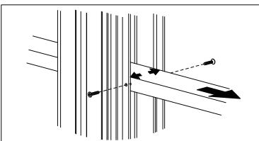
REMOVE THE SCREWS AND THE INSTALLATION SPACER.
