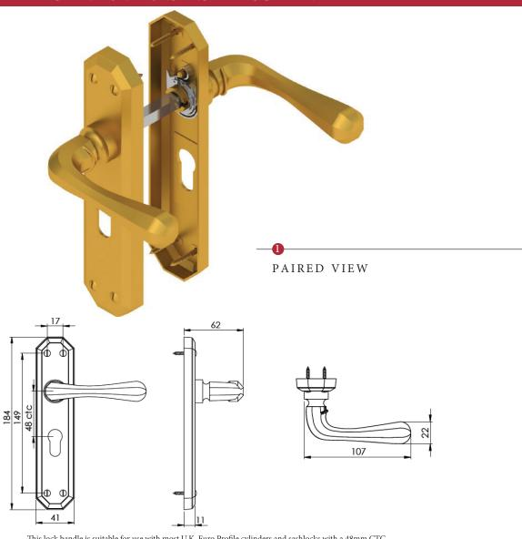
This lock handle is suitable for use with most U.K. Euro Profile cylinders and sashlocks with a 48mm CTC.
